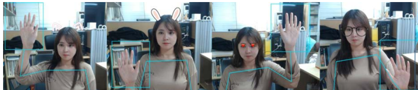
Fig.4 The system recognizes four types of classified 'Five' gestures and then shows the virtual object (that are from left to right: cat ear, rabbit ear, heart, and glasses).
